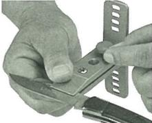
**PRO TIP:** For best results, the gap at the back of the clamp should be equal or *slightly* greater than the gap near the front jaws of the clamp. Approx. 5/8" of the blade should be exposed from the end of the clamp. *If the hone hits the thumbscrew, replace it with the flat head screw provided.* For blades approx. 1/2" and under wide, use the notch in the clamp. Position average or oversized blades beyond notch and well into the knife clamp (see diagram).
