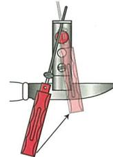
Start at the knife's base, near the guard and place the hone against the edge. Push the hone against the edge (into the blade), while moving the hone towards the tip of the blade covering a 2" section of blade per stroke. Lift the hone and repeat (always sharpen into the blade). Sharpen one side first, then flip entire clamp over and sharpen the opposite side using the same number of strokes on each side. For longer knives, sharpen in sections repositioning the clamp if needed.
